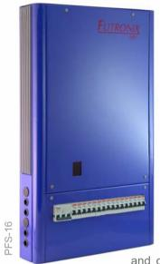
The PFS switching unit is available in 8, 12 or 16 channel formats and is designed for controlling dimmable fluorescent ballasts, curtain/drape/window shade motors and other motorized equipment such as swimming pool covers and sky lights. The unit has motor interlocking, for operating dual-motor curtain and drapes.
