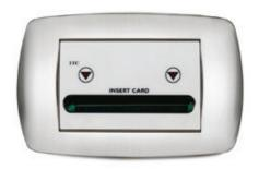
It detects the presence of guests or staff int he room and activates room services. It is provided with illuminated slot for ISO 7816 cards and two flashing leds for easier insertion. It is housed in 3-module box and connected to the UGC-M control unit by means of 6-wire cable terminated with RJ12 PLUG. Weight: 0.10 Kg. Depth 44mm.
