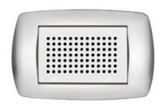
Small-size speaker for installation in 3-module box that is taken completely. The size of the loudspeaker permits a power of 3 W. Equipped with CA10MP amplifier module to be housed separately. Available in the series specified in the table. Weight: 0.16 Kg
