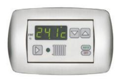
It allows the guest to change temperature, switch on and off the heating. The display shows time and set and measured temperature. The light sensor optimises contrast and luminous symbols give information on operation status. It is housed in 3-module box and connected to the control unit by means of 6-wire cable terminated with RJ12 PLUG. Weight: 0.10 kg. Depth 45mm.
