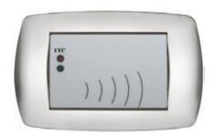
It provides access to common areas by proximity cards with ISO 7816 format in different mode for guests, visitors, manager, staff, maintenance operators, etc. Max. reading distance 5 cm. It is provided with 2 leds for card validity and one voltage free contact for door opening, with 24V, 4(2)A relay. It is housed in 3-module box and connected to the technological control unit UGT with 6-wire cable terminated with RJ12 PLUG. Weight: 0.1 kg. Depht: 53 mm.
