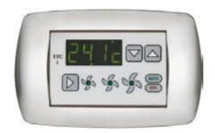
It allows the guest to change temperature, speed, automatic or manual operation and switch off air conditioning. The display shows time, set and measured temperature and speed. The light sensor optimises contrast and luminous symbols give information on operation status. It is housed in 3-module box and connected to the control unit by means of 6-wire cable terminated with RJ12 PLUG. Weight: 0.10 kg. Depth 45mm.
