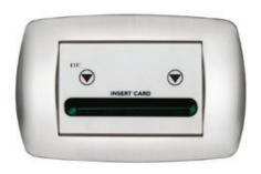
It detects the presence of guests or staff int he room by reading the inserted chip and activates room services only if the card is enabled. It is provided with illuminated slot for ISO 7816 cards and two flashing leds for easier insertion. It is housed in 3-module box and ocnnected to the UGC-M control unit by means of 6-wire cable terminated with RJ12 PLUG. Weight: 0.10 Kg. Depth 44mm.
