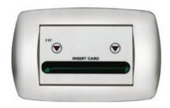
It detects the presence of guests and staff in the room and activates relevant services. It is provided with illuminated insertion slot for ISO 7816 cards and 2 flashing leds for easier insertion. It is housed in 3-module box and connected to the control unit Mega with 6-wire cable terminated with RJ12 PLUG. Weight: 0.1 kg. Depth 44mm.
