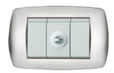
It measures the temperature of the room where it is installed. It is composed of an NTC sensor and is installed in a standard blank insert. It must be installed at 150/170 cm from the ground, in specific box away from heat sources or air draughts. Weight: 0.03 kg. Depth 35mm.
