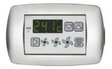
It allows the guest to change temperature, speed, automatic or manual operation and switch off air conditioning. The display shows time, set and measured temperature values and speed. The light sensor optimises contrast and luminous symbols provide information on operation status. It is housed in 3-module box and connected to the control unit by means of 6-wire cable terminated with RJ12 PLUG. Weight: 0.1 kg. Depth: 45mm.
