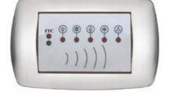
It provides access to the room in different mode for guests, managers, staff and maintenance operators. It is provided with illuminated insertion slot for chip cards with ISO 7816 format and 2 leds for card validity. It is also provided with 5 light signals to display: "guest in room", "do not disturb", "room to clean", "mini-bar to check", "help call/flood". It is housed in 3-module box and connected to room activator with 6-wire cable terminated with RJ12 PLUG. Weight: 0.1 kg. Depth 50mm.
