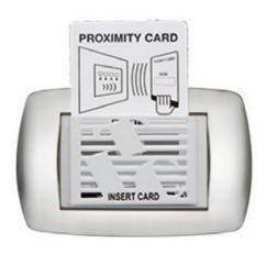
It detects the presence of guests or staff in the room by reading the proximity card inserted in the external pocket and activates room services only if the card is enabled. It is provided with 2 flashing leds for easier insertion. It is housed in 3-module box and connected with Mega control unit with 6-wire cable terminated with RJ12 PLUG. Weight: 0.1 kg. Depth 50mm.
