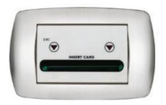
It detects the presence of guests or staff in the room by reading the inserted chip and activates relevant services only if the card is enabled. It is provided with illuminated insertion slot for ISO 7816 cards and 2 flashing leds for easier insertion. It is housed in 3-module box and connected to the control unit Mega with 6-wire cable terminated with RJ12 PLUG. Weight: 0.1 kg. Depth 50mm.
