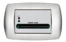
It provides access to common areas in different mode for guests, visitors, manager, staff, maintenance operators, etc. It is provided with illuminated insertion slot for chip card with ISO 7816 format, 2 leds for card validity and one voltage free contact for door opening with 24V, 4(2)A relay. It is housed in 3-module box and connected to the technological control unit UGT with 6-wire cable terminated with RJ12 PLUG. Weight: 0.1 kg. Depht: 50 mm.
