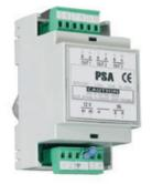
It amplifies incoming signal and splits it over three different outputs. It is housed in 3-module box for DIN rail. 12Vac, 15VA power supply. Dimensions (lxhxd): 54x96x58 mm. Weight 0.1 kg.
