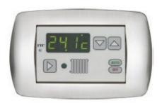
It allows the guest to change temperature and switch on and off the heating. The display shows time, set temperature and measured temperature. The light sensor optimises contrast and luminous symbols provide information on operation status. It is housed in 3-module box and connected to the control unit by means of 6-wire cable terminated with RJ12 PLUG. Weight: 0.1 kg. Depth: 45mm.
